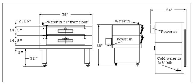
Electrical: 208/220 Volt 3 Phase 60 Hz 56 Amps 20 Kw. Recommend a slow-blow breaker\*
