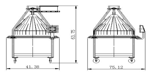
Electrical: 208/220 Volt 3 Phase 60 Hz 10 Amps. Supplied with Twist-Lock plug # L15-20P
