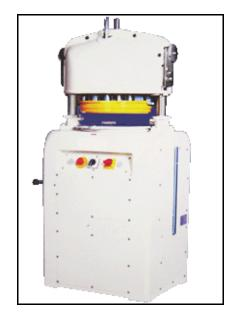
Electrical: 208/220 Volt 3 Phase 60 Hz 8 Amps Standard. Supplied with twist lock plug ( P & S L1520P ). Recommend a 15 amp slow blow breaker. Other voltages and phases available upon request.
