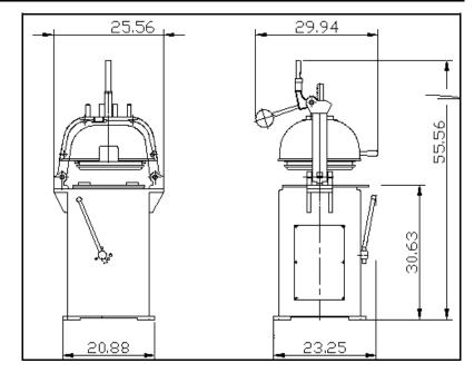
Electrical: 208/220 Volt 3 Phase 60 Hz 4 Amps Standard. Supplied with twist lock plug (P & S L1520P). Recommend a 10 amp slow blow breaker. Other voltages and phases available upon request.
