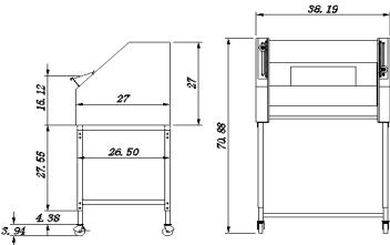
Electrical: 208/220 Volt 3 Phase 60 Hz 8 Amps. Supplied with Twist-Lock plug # L15-20P
