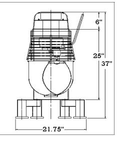
Electrical: 115 Volt 1 Phase 60 Hz 12 Amps 1.5 HP. Supplied with grounding plug.
