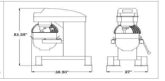
Electrical: 208/220 Volt 3 Phase 60 Hz 8 Amps 2 HP. Supplied with Twist-Lock plug.
