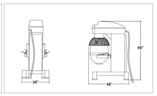
Electrical: 208/220 Volt 3 Phase 60 Hz 16 Amps 5 HP. Supplied with twist-lock plug.
