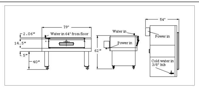
Electrical: 208/220 Volt 3 Phase 60 Hz 28 Amps 10 Kw. Recommend a slow-blow breaker\*
