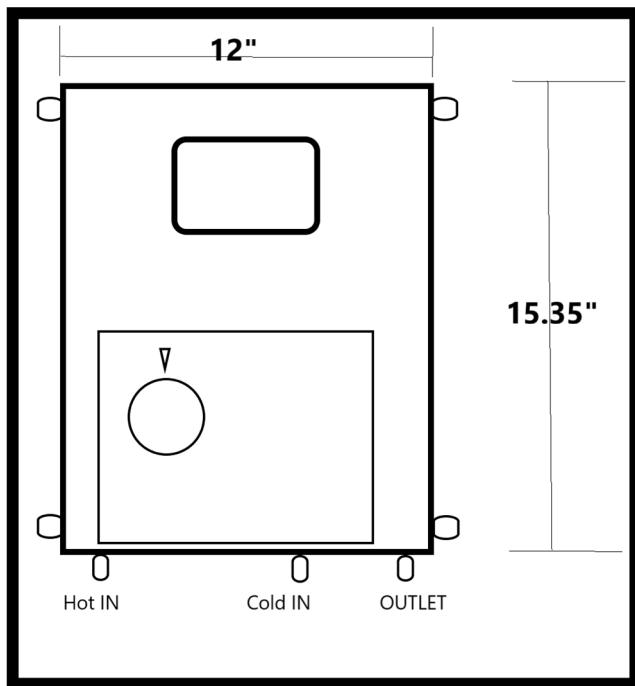
Electrical: 115 Volt 1 e 60 Hz 1.2 Amps. Supplied with grounding plug NEMA L520P
