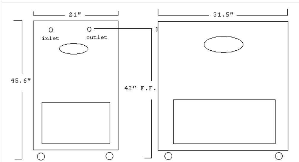
**Electrical:** 208/220 Volt, 1 Phase, 60 Hz 7 / 6 Amps, 1 kW. 6-foot cord with twist-lock plug. 2 wire + ground (NEMA plug: L620P) Recommend a 15 Amp breaker.
