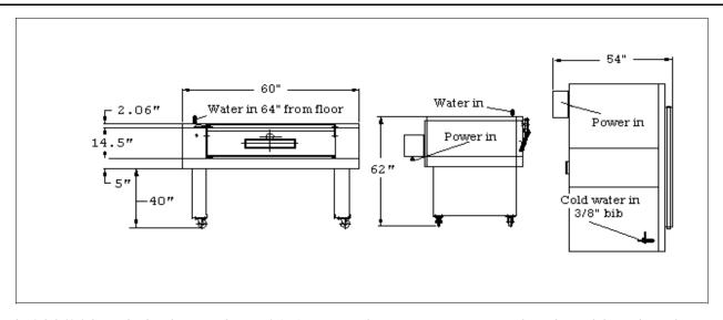
Electrical: 208/220 Volt 3 Phase 60 Hz 21 Amps 7.4 Kw. Recommend a slow-blow breaker
